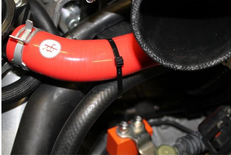
14. The last step is to connect the hose from the Cam Cover to the T. Trim the hose if necessary and secure with a hose clamp.
