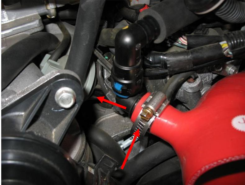
11. Insert the plug included with the VTA kit in to the intake hose and secure it with the clamp removed in step 10.
