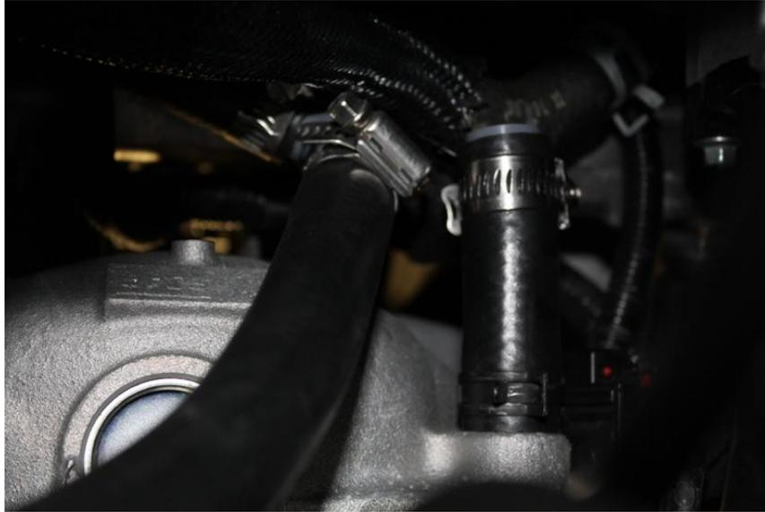
10. Remove the OEM hose from the CAM cover by squeezing the 2 green tabs and pulling the hose off of the cam cover. Then, remove the green clip from the Cam Cover.
