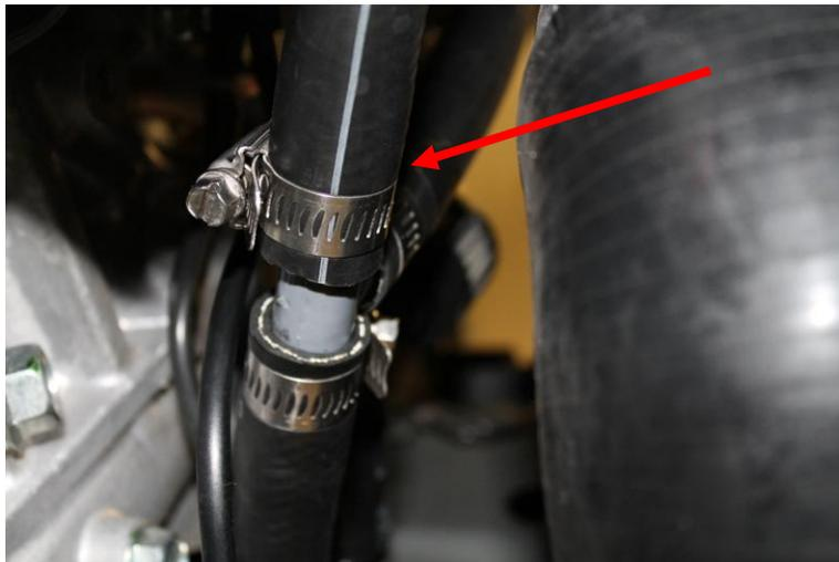
9. Attach the short hose and plug included with the VTA kit to the intake manifold port.
