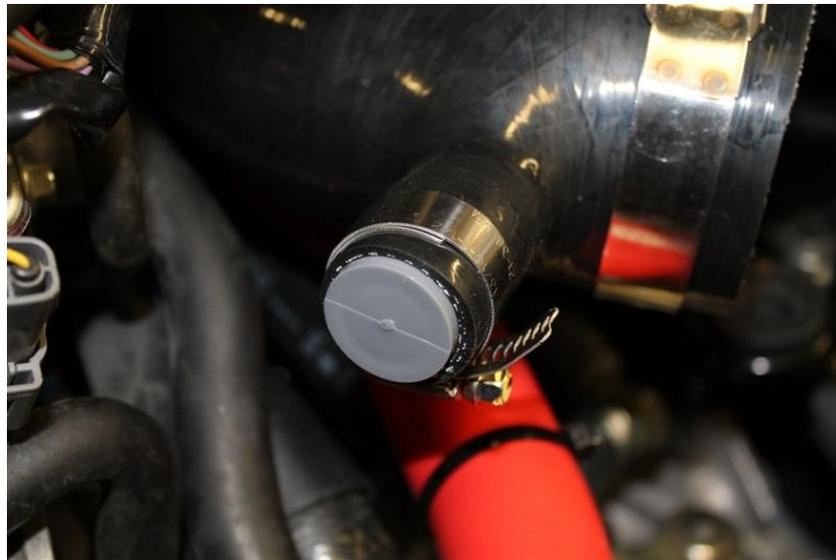
12. Next, feed the other hose removed in step 7, down in front of the EGR valve, underneath the bypass hose and connect it to the cam cover vent with a hose clamp. **This can be done without removing the battery box. The picture below illustrates the routing if the battery box and turbo inlet pipe was removed.**
