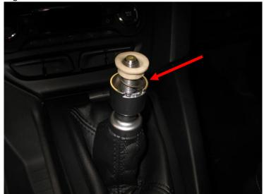
3. Remove the shift boot surround by either slipping a trim tool between it and the base of the console or using your hands. It is held in place by 4 clips that will need to be popped apart. Some effort is required to separate it. Do not bend the surround too much.
