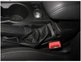
14. Pull the boot inside out and slide boot and cover off the emergency brake. Return the boot to right side out for reinstallation later.
