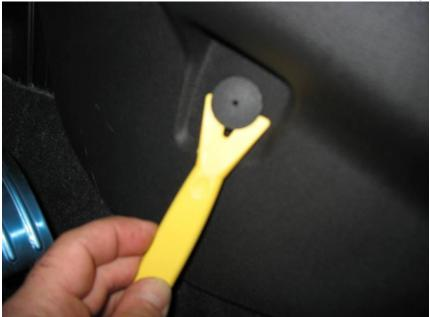
6. Separate the rear lower portion of the kick panel from the main portion of the console. Then begin separating it by moving up and towards the front of the vehicle. Separate it completely from the adjoining change cup but do not remove it completely from the vehicle.
