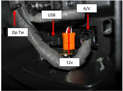
18. With everything now disconnected, remove the console by pivoting the front up. Make sure the emergency brake is all the way up providing clearance. Remove the console from the vehicle.
