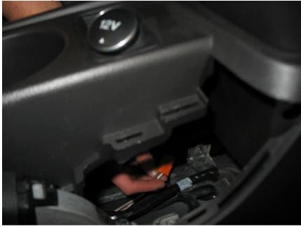
17. From the driver's side back seat, hold the console up and remove the rear 12v accessory connector by pulling it straight off. Remove the USB connector by squeezing the tab and pulling it off. And remove the A/V connector by squeezing the tab and pulling it off. There is also a zip tie securing the wiring loom to the console that must be clipped.
