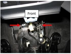
20. Using a screwdriver, pry the sleeves of the OEM shifter bushings out. Then push the rubber grommet portion out through the bottom of the shifter base.
