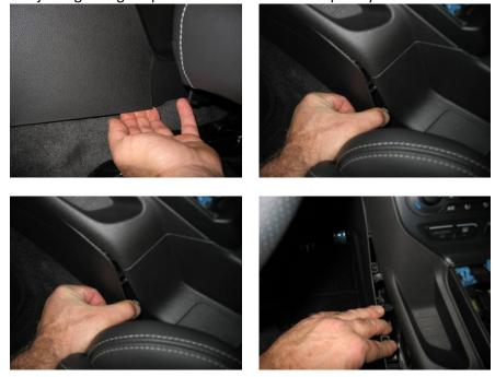
7. On the passenger's side, remove the small cover to expose the christmas tree fastener and then remove the fastener.
