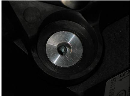
22. Place a washer on top of each and reinstall the 2 front bolts removed in step 19. Only finger tighten them for now.
