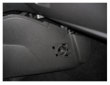
9. Using a 7/32 or 5.5mm socket, remove the three screws shown below.
