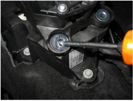
21. With all 4 sleeves and bushings removed in step 20, now install your new JBR Solid Shifter Base Bushings. Install the front 2 first. They should be installed with the smaller diameter side up and properly indexed in to the bottom of the shifter base.
