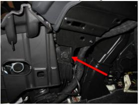
13. Remove the emergency brake cover and boot by pulling up on the front corner. Pivot the cover towards the rear of the vehicle to remove the rear portion of the cover.
