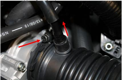
3. Next remove the lead connected to the MAF sensor by depressing the tab at the rear of the connector then, pull the connector towards the rear of the car.
