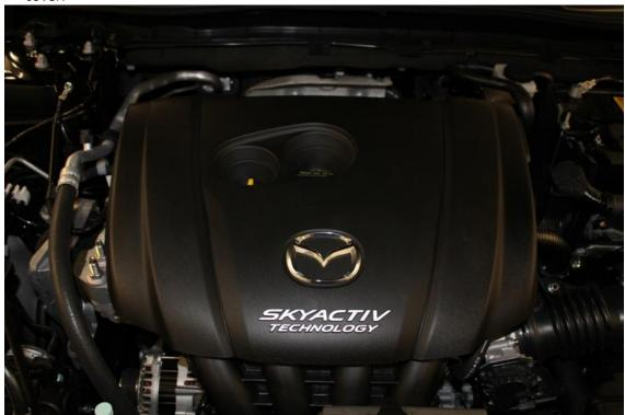
2. With a Philips head screw driver, loosen the hose clamp at the throttle body and remove the cam cover vent tube by pulling straight up.
