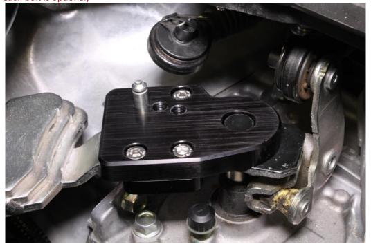
20. Install the linkage pin in the desire location and tighten with a ¼" open end wrench. (One drop of loctite on the pin is optional)
