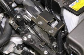
19. Place the top half of the JBR short shift arm adapter over the OEM linkage pin and on to the OEM shifter arm. Position the bottom half below the arm and secure using the 3, 6mm x 14mm bolts included with your kit. Tighten evenly using a 5mm allen wrench. (One drop of loctite on each bolt is optional)
