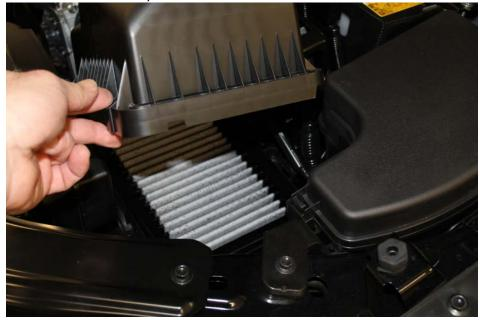
6. Using a razor knife carefully cut the tape securing the MAF sensor wire from the back of the air box cover and remove the cover from the vehicle.
