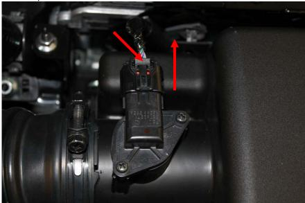
4. Unclip the 2 clips holding the air box cover in place
