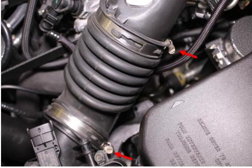
7. Remove the valve cover vent tube from the rear of the OEM intake by squeezing the connector and pulling towards the rear of the vehicle.
