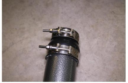
11. Being careful not to scratch the intake, lay it on its side, slide it under the cowl, rotate the turbo end down and the other end over towards the driver's side keeping it up and clear of anything on the top of the engine that could scratch it. The next series of pictures illustrates how to do it.
