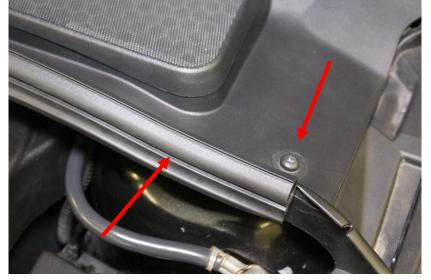
2. Remove the four plastic button fasteners across the front of the cowl using a flat head screwdriver to remove the cap then the base.
