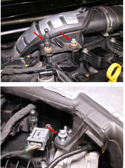
6. Using a 10mm socket loosen both clamps securing the OEM induction hose.
