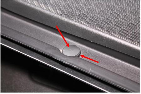
3. Remove the two 10mm bolts on both sides of the cowl found beneath the outer cover. Remove the cowl from the vehicle.
