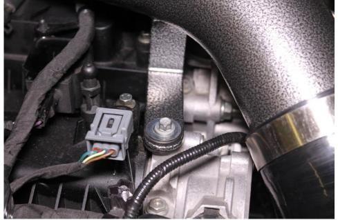
16. Re-install the post used to hold the engine cover.
