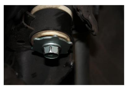
7. Pull down on the sub-frame as much as possible and remove the bolts securing the OEM sway bar brackets with a 14mm Socket.
