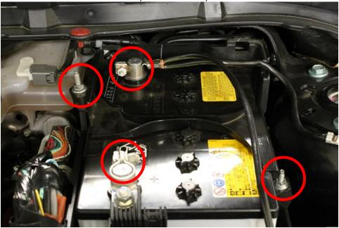
10. Remove the three 10mm bolts in the bottom of the battery box .
