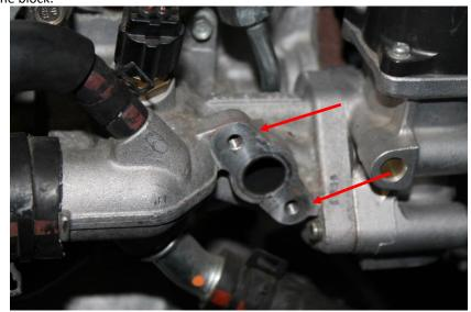
19. Apply gasket sealant (Red RTV) to one side of the EGR plate, add the factory gasket found on the flange of the OEM EGR tube, Re-install with the two bolts removed in step 18 and tighten.
