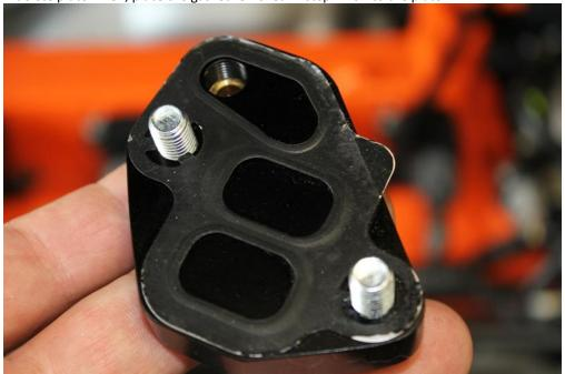
25. Install the EGR plate on to the motor. Using a 12mm socket, tighten the bolts to 10ftlbs. Reinstall the coolant line using the supplied clamp.
