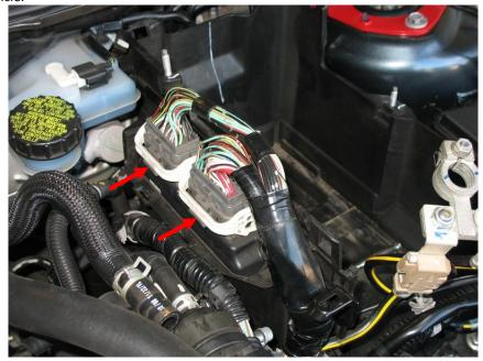
12. Remove the two 10mm nuts securing the wiring harness bracket. Lift the bracket off the studs and lay wiring harness over towards the front driver's side so it's not in your way.
