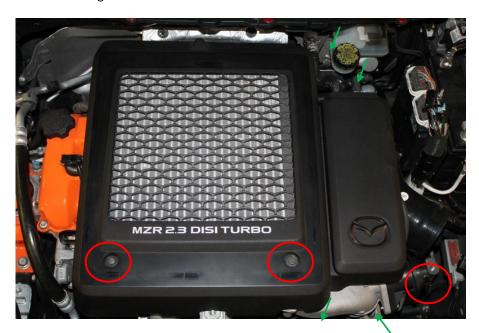
2. Using a philips head screwdriver, loosen the clamp securing the intake tube to the top of the factory air box. Then remove the connection to the MAF sensor by squeezing the tab and pulling the connector off.
