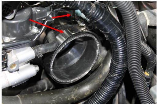
19. Next remove the OEM rubber grommet used to secure the OEM turbo inlet pipe the motor and install it on to your new intake.
