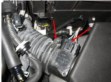
3. Unclip the fasteners securing the top the air box to the bottom
