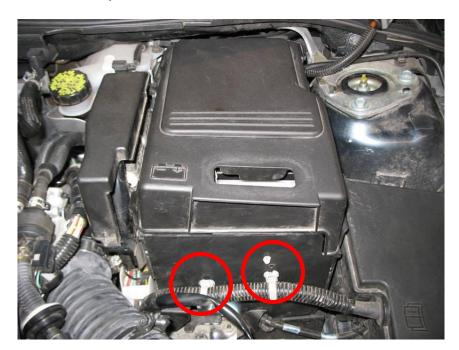
12. Remove the three 10mm bolts in the bottom of the battery box.
