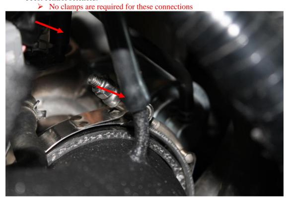
22. Cut approximately 6" off the 5/8" silicone hose included with your kit and install the 90 degree barbed adaptor on to one end. Add the remaining hose to the other leg of the 90 degree barbed adaptor. Install the long hose on to the valve cover vent and the short end on to the intake adjusting the length of the hoses as needed.
