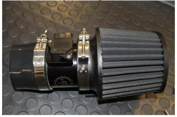
26. Add the remaining T-bolt clamp included with your kit to the end of the MAF coupler and slip the MAF housing and filter assembly on to the intake. Adjust the MAF housing and filter assembly as needed and tighten the T-bolt clamp with a 10mm socket.
