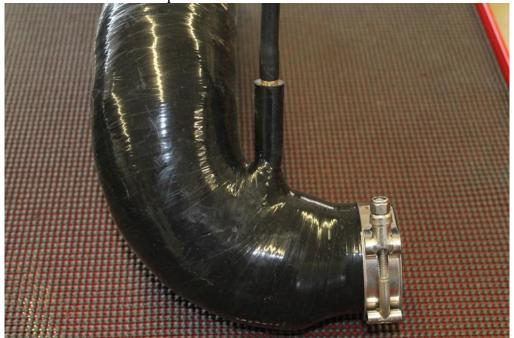
24. Now install your new JBR Wide Path Intake System in to the vehicle, on to the turbo inlet. Locate the mounting clamp on to the factory mounting location and secure it with the 10mm nut removed in step 16. Tighten the clamp at the turbo
