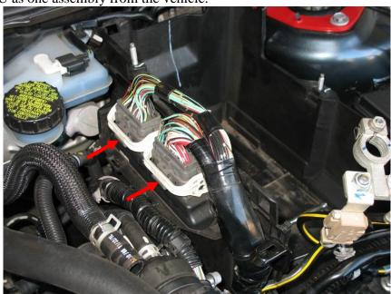
14. Remove the two 10mm nuts securing the wiring harness bracket. Lift the bracket off the studs and lay wiring harness over towards the front driver's side so it's not
