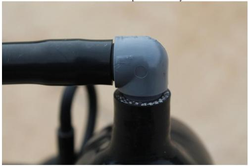
21. Insert the aluminum silicone joiner in to the recirculation tube and secure with the included clamp. For non-recirculation applications insert the included plug and secure with the included clamp.
