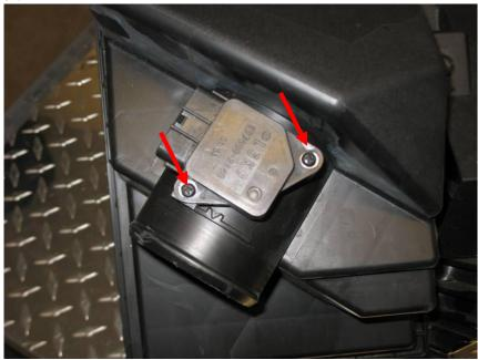
30. Place one included T-bolt clamp on to the intake, insert the MAF housing as shown and tighten the clamp with a 10mm socket.
