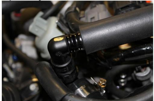
26. If you're installing the 3.5" intake, remove the OEM valve cover hose from the valve cover suing the same method as in step 17. Then, connect the silicone hose from the intake to the valve cover.
