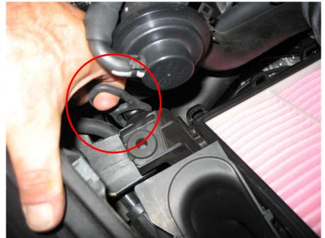
8. Tug up on the bottom of the air box and remove it from the vehicle.
