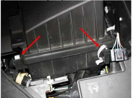
4. Lift the top of the air box up, push the intake hose off and remove the top of the air box from the vehicle.
