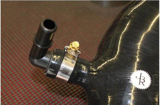
20. If you're installing a 3.5" intake, install the included 90 degree fitting and silicone hose in to the intake as shown. No clamps are necessary for these connections.
