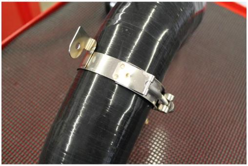
23. Place one included T-bolt clamp on to the intake and insert the vacuum line in to the little black vacuum port.
