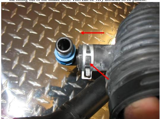
19. If you're installing the 3" intake system insert the fitting removed in step 18 in to your new JBR Wide Path Intake and secure it with the included clamp.
