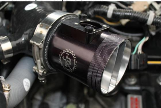
31. Install the MAF sensor in to your new JBR MAF housing using the 2 socket cap screws included with your kit. Then tighten with a 3mm allen wrench.
