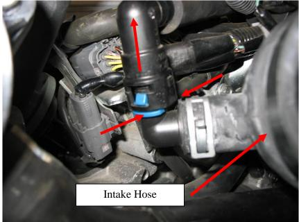
18. Orient the included T-bolt clamp on to your new JBR Turbo Inlet Pipe as shown below, slip the turbo inlet mounting bracket under the T-bolt camp just slightly off center and tighten the T-bolt clamp.
