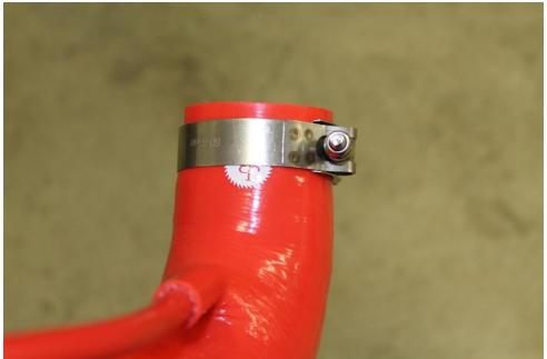
20. Install the turbo inlet pipe on to the turbo. Slide the turbo inlet mounting bracket on to the stud and reinstall the 10mm nut removed in step 16. Tighten the T-bolt
