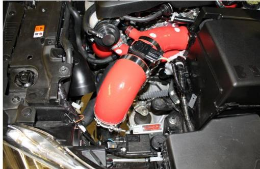
12. It may be necessary to bend the tab down on the cover of the fuel pump resistor shown below to make clearance for the cold air pipe.
