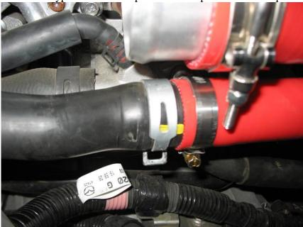
23. Using a pair of pliers squeeze the silver clamp securing the 90 degree valve cover breather fitting to the intake hose and pull the fitting out of the intake hose. This can be very difficult so be patient.
