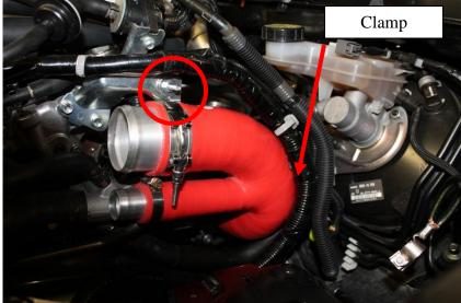
21. Connect the new vacuum line included with your turbo inlet pipe to the boost
