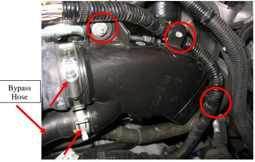
17. Disconnect the valve cover breather connection from the 90 degree fitting in the intake hose by squeezing both blue tabs together then pulling up. Then remove the intake hose and turbo inlet pipe as one assembly from the vehicle.
