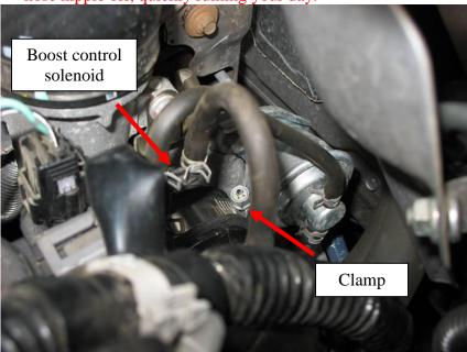
16. Use a pair of pliers to squeeze the clamp securing the bypass hose to the turbo inlet pipe and slide it towards the front of the vehicle, then remove the bypass hose from the turbo inlet pipe. Using a 10mm socket remove nut circled below. Using a pair of needle nose pliers, remove the 2 fasteners securing the wiring harness to the turbo inlet pipe.
