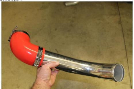
11. Slip the pipe down in to the engine bay so the cold air pipe extends in to the wheel well area. Slide the elbow on to the end of the MAF housing up to the end of the
