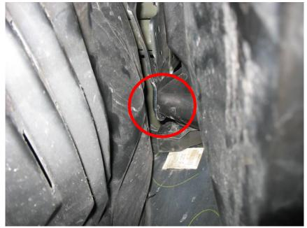
6. Remove the push pin fastener securing the cover to the frame. A flat heat screw driver works well for removing the center portion of the push pin fastener.
