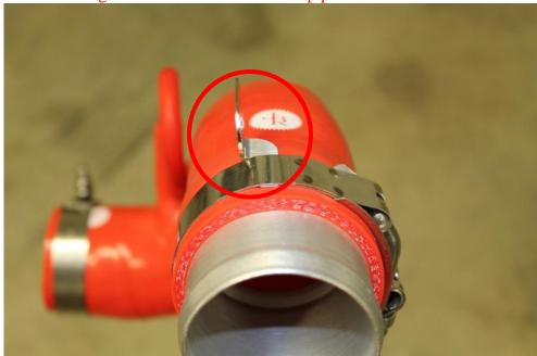
19. Place the included T-bolt Clamp on to your JBR turbo Inlet Pipe and orient as shown below.
