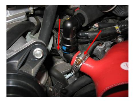
32. Using a philips head screwdriver, remove the MAF sensor from the factory air box cover.
