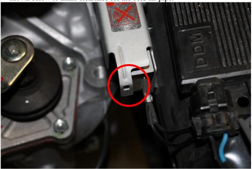
13. Place the included worm clamp over the end of the cold air pipe, loop it over the bracket installed in step 45 and tighten the clamp.
