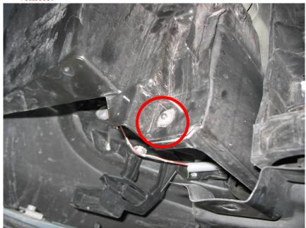
8. Drill in 1/8" hole then a 1/4" hole the forward most tab in the frame.
