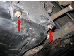
4. Remove the three philips head screws holding the front potion of the driver's side inner fender liner to the lower portion of the bumper and fold it towards the rear of the vehicle out of your way.
