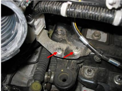
15. Using a pair of needle nose pliers, squeeze the clamp on the boost control solenoid vacuum hose and slide it up. VERY, VERY CAREFULLY twist the hose to loosen the it from the boost control solenoid and remove the hose. Using a philips head screwdriver, loosen the clamp securing the intake hose to the turbo inlet pipe.
