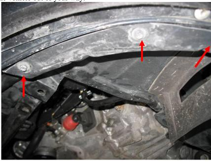
5. Up high in front of the driver's side inner fender well is a 10mm bolt securing a plastic cover that need to be removed. Denting in the fender well will help to get the socket wrench in between.
