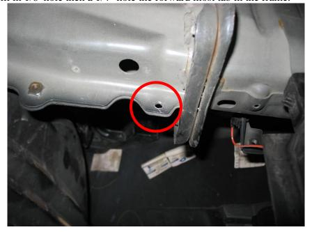
9. Install the mounting bracket include with your cold air kit as shown using the 6mm bolt, flat washer, lock washer and nut also included. Then tighten with a 10mm socket and 10mm wrench
