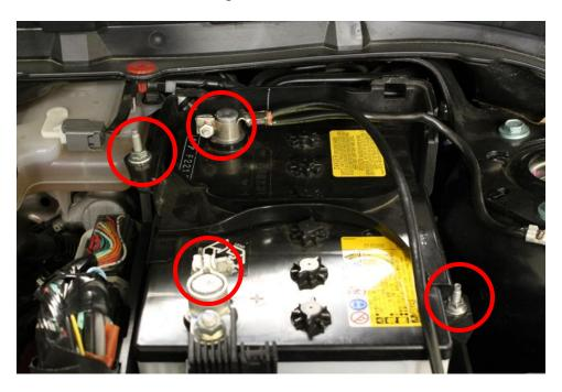
11. Using a pair of needle nose pliers remove the fasteners securing the wiring harness to the front cover of the battery box. There are two on the outside and one inside. Slide the front cover of the battery box up and remove from the vehicle. Remove the battery.
