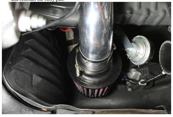
15. Using a 10mm socket tighten the two clamps on the silicone elbow.
