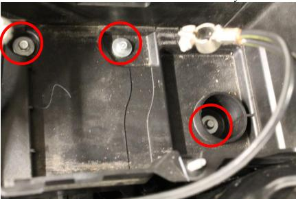
13. Disconnect the wiring harness from the ECU by pressing the tab below the white handle. Then lift the handle to remove the connector. Remove the battery box and ECU as one assembly from the vehicle.
