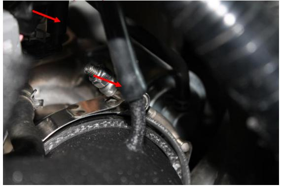
20. Cut approximately 6" off the 5/8" silicone hose included with your kit and install the 90 degree barbed adaptor on to one end. Add the remaining hose to the other leg of the 90 degree barbed adaptor. Install the long hose on to the valve cover vent and the short end on to the intake adjusting the length of the hoses as needed.
