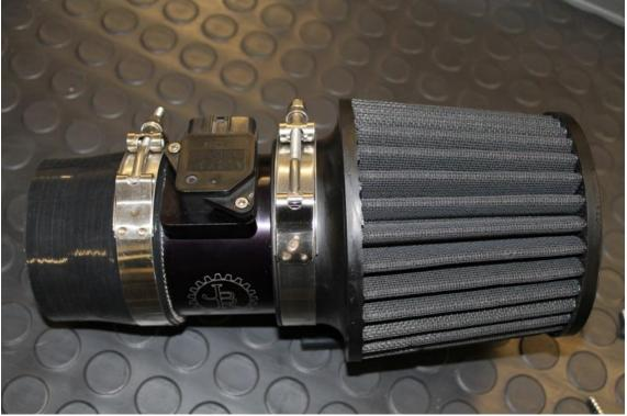
24. Add the remaining T-bolt clamp included with your kit to the end of the MAF coupler and slip the MAF housing and filter assembly on to the intake. Adjust the MAF housing and filter assembly as needed and tighten the T-bolt clamp with a 10mm socket.
