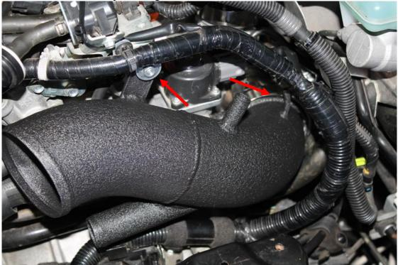
19. Install the included boost control solenoid vacuum line on to the intake and the boost control solenoid.
