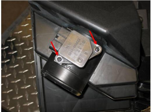
23. Install the MAF sensor using the included screws and tighten with a 3mm allen wrench. Install the JBR Dry Flow Filter and MAF coupler and secure both with the included T-bolt clamps as shown and tighten with a 10mm socket.
