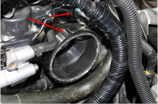
17. Next remove the OEM rubber grommet used to secure the OEM turbo inlet pipe the motor and install it on to your new intake.
