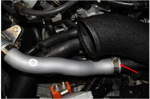
22. Remove the MAF sensor from the factory air box using a philips head screw driver.
