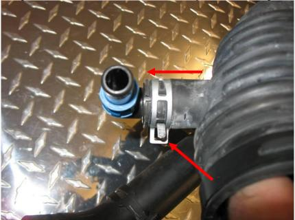
17. If you're installing the 3" intake system insert the fitting removed in step 16 in to your new JBR Wide Path Intake and secure it with the included clamp.
