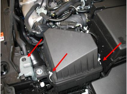
4. Lift the top of the air box up, push the intake hose off.
