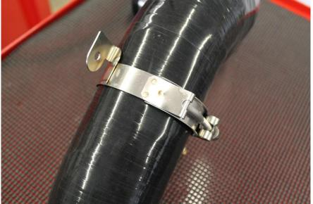
21. Place one included T-bolt clamp on to the intake and insert the vacuum line in to the little black vacuum port.
