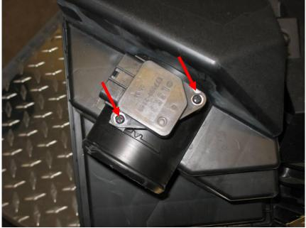
28. Place one included T-bolt clamp on to the intake, insert the MAF housing as shown and tighten the clamp with a 10mm socket.
