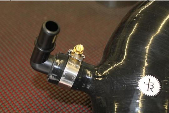
18. If you're installing a 3.5" intake, install the included 90 degree fitting and silicone hose in to the intake as shown. No clamps are necessary for these connections.
