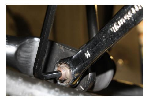
2. Using a 10mm socket and a 14mm socket, remove the cross member.
