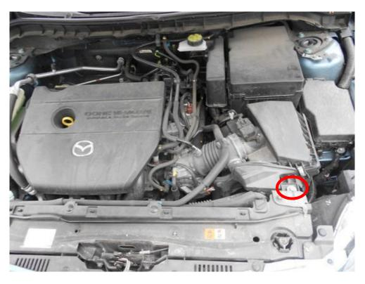
3. Remove the MAF sensor connector by depressing the tab at the rear of the connector and pull towards the rear of the vehicle.
