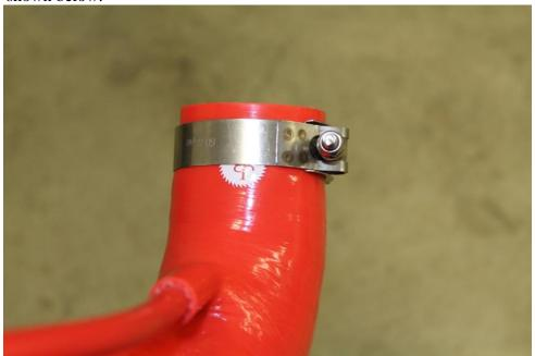
18. Install the turbo inlet pipe on to the turbo. Slide the turbo inlet mounting bracket on to the stud and reinstall the 10mm nut removed in step 14. Tighten the T-bolt
