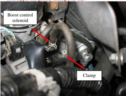
14. Use a pair of pliers to squeeze the clamp securing the bypass hose to the turbo inlet pipe and slide it towards the front of the vehicle, then remove the bypass hose from the turbo inlet pipe. Using a 10mm socket remove nut circled below. Using a pair of needle nose pliers, remove the 2 fasteners securing the wiring
