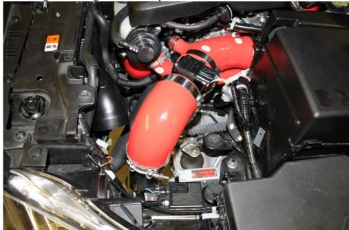
9. It may be necessary to bend the tab down on the cover of the fuel pump resistor shown below to make clearance for the cold air pipe.
