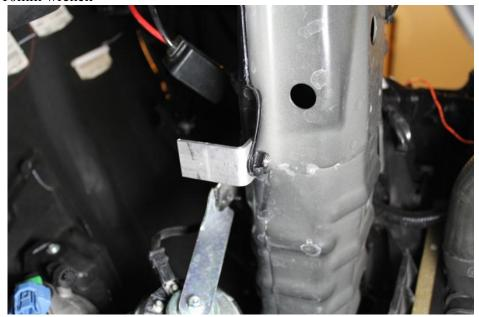
7. Remove your JBR Dry Flow filter from the end of the MAF housing using a 10mm deep socket. Place 2 T-bolt clamps included with your Stage 3 kit on to the silicone elbow. Slip the elbow on to the cold air pipe and orient the elbow as shown below.
