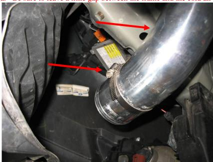
11. Reinstall your JBR Dry flow filter, replace the front portion of the fender liner and reinstall the belly pan.
