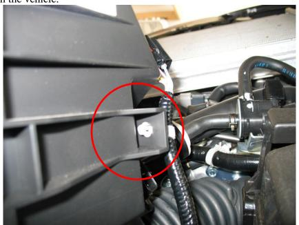
6. Tug up on the bottom of the air box remove it from the vehicle.
