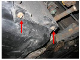
4. Remove the three philips head screws holding the front potion of the driver's side inner fender liner to the lower portion of the bumper and fold it towards the rear
