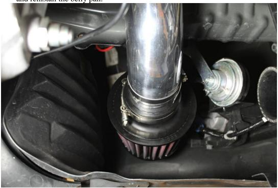
12. Using a 10mm socket tighten the two clamps on the silicone elbow.
