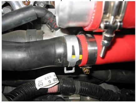
21. Using a pair of pliers squeeze the silver clamp securing the 90 degree valve cover breather fitting to the intake hose and pull the fitting out of the intake hose. This
