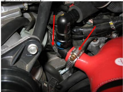
31. Using a philips head screwdriver, remove the MAF sensor from the factory air box cover.
