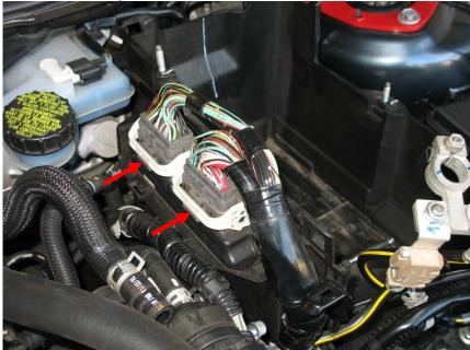
12. Remove the two 10mm nuts securing the wiring harness bracket. Lift the bracket off the studs and lay wiring harness over towards the front driver's side so it's not
