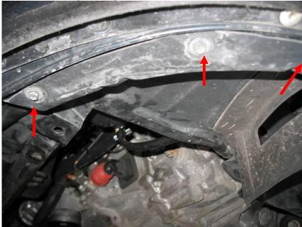
5. On the driver's side, remove the 10mm bolt from the forward most tab in the frame.
