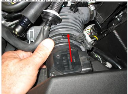
5. Remove the grey wire connector from the top section of the air box and remove from the vehicle.
