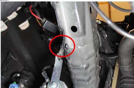
6. Install the mounting bracket include with your cold air kit as shown using the 6mm bolt, flat washer, and lock washer. Then tighten with a 10mm socket and 10mm wrench
