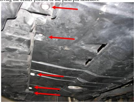
3. There are four more 10mm bolts located near the wheels; two on each side.
