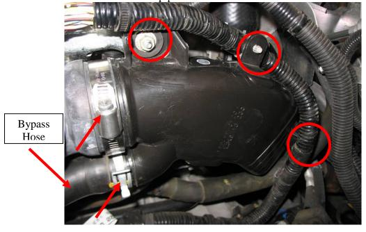
15. Disconnect the valve cover breather connection from the 90 degree fitting in the intake hose by squeezing both blue tabs together then pulling up. Then remove the
