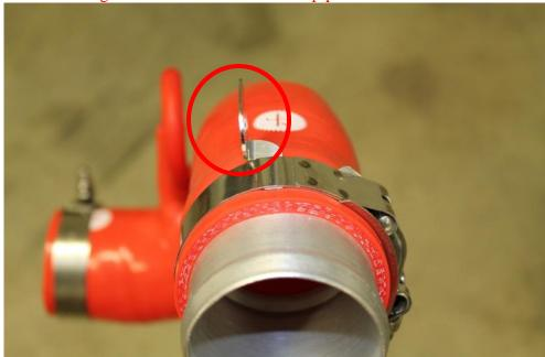
17. Place the included T-bolt Clamp on to your JBR turbo Inlet Pipe and orient as shown below.
