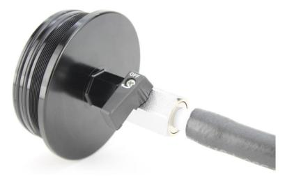
3. Apply Teflon tape to the threads of the barbed fittings. Install the barbed fittings into the IN and OUT ports of the catch can using a 17mm deep socket.
