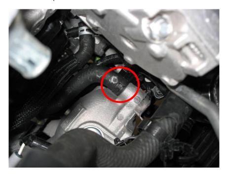
10. Now remove hose from the PCV valve. This is the most difficult to remove and will take some time. Be careful not to tug/yank too much on the hose; the PCV valve fitting is made of plastic. Remove the hose from the engine and save both clamps.
