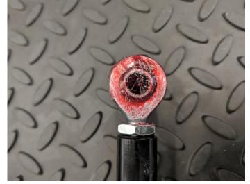
4. Install the upper and lower ends of your new JBR Adjustable Front End Links on to the sway bar and strut then tighten with a 17mm wrench.
