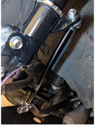
5. Adjust the length of the end links as needed and tighten the jam nuts.
