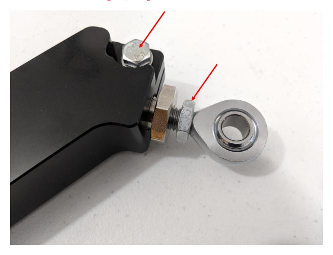
7. Install your new JBR camber arm back in the car. The bushing end should be inboard and the rod end should be out by the wheel. Using 2 of the spacers provided, locate one spacer on each side of the rod end for the outer ends of the camber arm only. Tighten both ends to 55ft/lbs.
