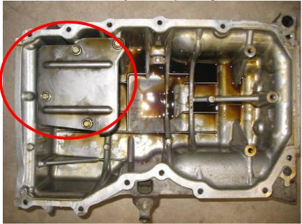
11. Install your new JBR Oil Pan Baffle kit as shown. Re-use the 4 bolts removed in step 11 and 2 included with the baffle kit. Tighten all 5 bolts to 18ft/lbs.
