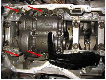
8. Put a little oil to the o-ring of your new JBR Balance Shaft Delete Kit. Apply some red or blue Loctite to the supplied bolt; add the washer and install as shown below.
