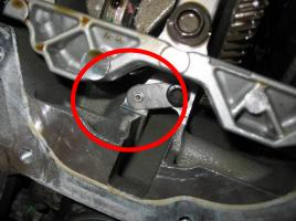
9. Re-install the oil pick up tube removed in step 7.
