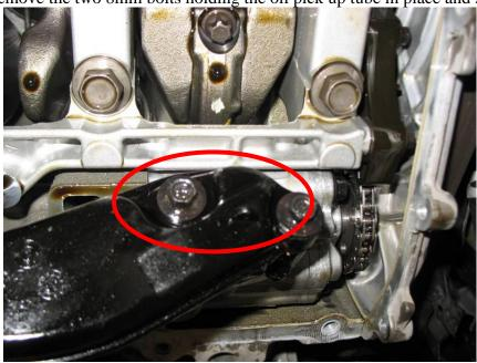
7. Remove the 4 balance shaft assembly bolts using a 14mm socket..
