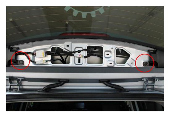
To remove the tray cable holders pull the center pin out and remove the fastener.
