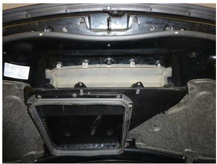
2. Put the hood scoop insert in place over the two center nuts. Make sure the bottom portion of the insert is above the two tabs in hood on both sides.
