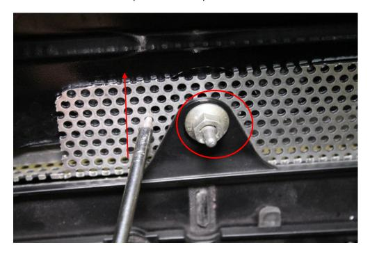
4. Close the hood and ensure that the insert is up behind the lip in the top of the hood scoop. If it's not, use gentle pressure to push it back until it's behind the lip. Push only in the center and just left or just right of center. DO NOT push far right or far left.
