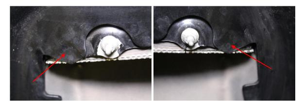
3. Once the insert is properly in place above the tabs, put a pick through one of the holes near a nut that secures it and use the pick to push the insert towards the front of the hood. While holding the insert forward, tighten the nut that secures the scoop insert. Do this for both nuts then reinstall the other two nuts that secure the scoop removed in step 1.
