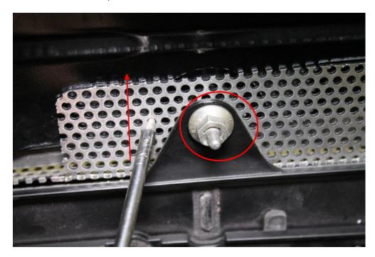
5. Next, tighten all remaining nuts left loose in step 3 and install the three plastic push pins removed in step 1.
