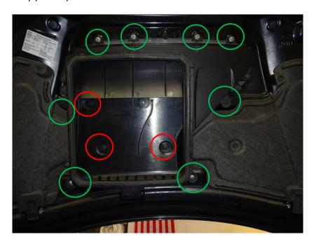
2. Put the hood scoop insert in place over the two center nuts. Make sure the bottom portion of the insert is above the two tabs in hood on both sides.
