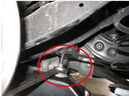
4. Apply 1 complete packet of grease in to each of the new included sway bar bushings and slip the bushings over the sway bar. Place the brackets on to the bushings. The grease provided is for initial installation and bushing break in. Additional grease will be required. The use of synthetic ONLY grease is recommended.
