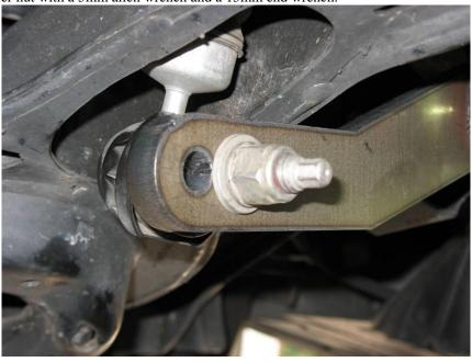
6. Put 1 drop of Loctite on each of the 4 sway bar bushing bracket bolts and loosely install each of them through the new bushing brackets securing the sway bar to the vehicles sub-frame
