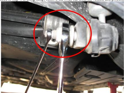
3. Using a 5mm allen wrench and 15mm end wrench remove the top nut off only one of the end links. Remove the end link and the sway bar from the vehicle.
