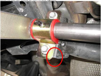
8. Tighten both of the nuts on each of the end links.
