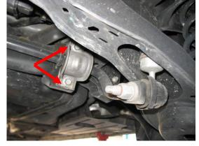
2. Using both a 8mm and 18mm wrench remove 2 nuts from both end links. If using jack stands proceed to step 4. If using ramps remove the sway bar from the vehicle and proceed to step 5.
