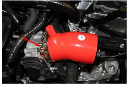
12. Insert the hose from the cam cover in to the vent port on the silicone hose.
