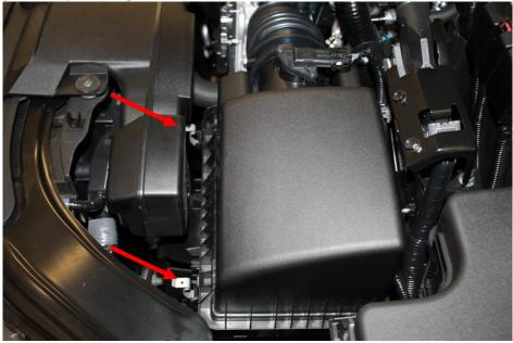
5. Separate the top of the air box from the bottom and remove the rubber accordion hose attached to the throttle body.
