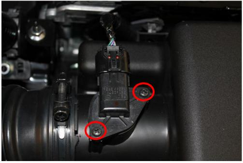
10. Now insert the sensor in to your new JBR MAF housing and secure it will a 3mm allen wrench.
