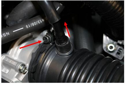
3. Next remove the lead connected to the MAF sensor by depressing the tab at the rear of the connector and pull the connector towards the rear of the car.
