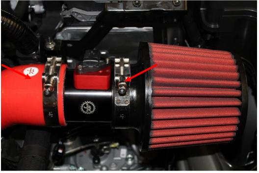
14. Re-connect the MAF sensor wire to the sensor. You will hear is snap when properly connected.
