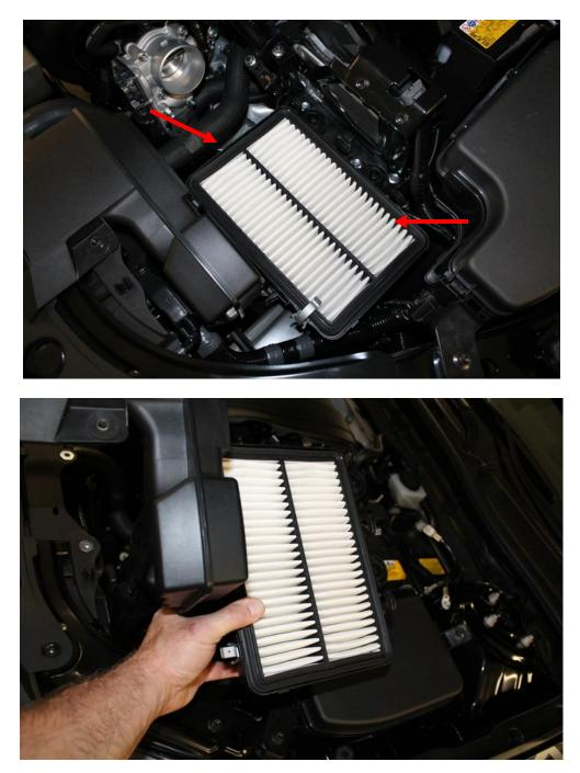
8. The next step is to grab the bottom section of the air box firmly and give it a swift tug upwards to remove the entire lower portion of the air box from the vehicle.
