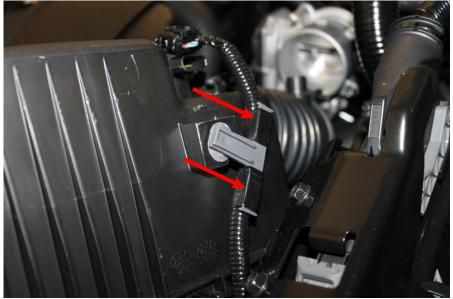
7. Using a 10mm socket remove the two bolts shown below.
