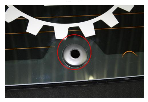
8. Put the lock washer on the 6mm bolt, slip it through the inner cap and put the rubber washer over the bolt. Put the outer cap in place and hold it with one hand. Close the hatch part way and look inside to center the outer cap with the hole in the glass. The o-ring should not be visible. Once the outer cap is centered and the logo is straight, thread the inner cap into the outer cap.
