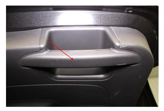
2. Using a 7mm socket remove the two bolts under each handle cover.
