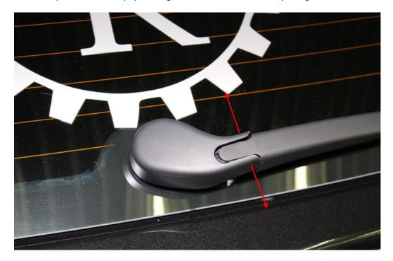
5. Use a 13mm socket to remove the wiper arm retaining nut. Wiggler the arm to remove it .
