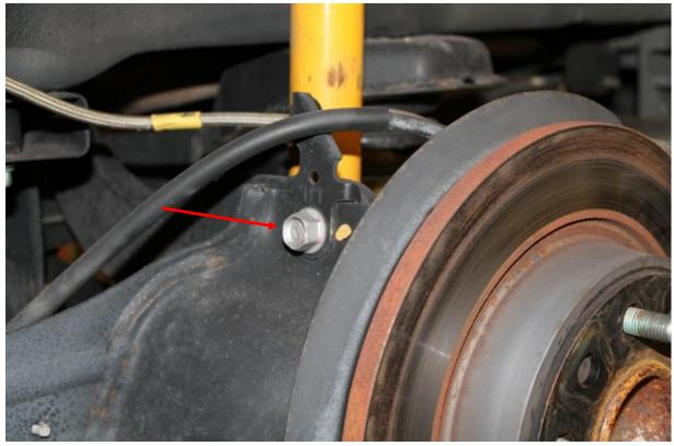
3. Using a 15mm socket or 15mm wrench remove the bolt securing the inner end of the OEM camber arm.
