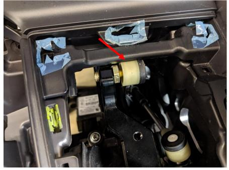
40. Check and insure that you can access all gears. If you experience difficulty perform <u>the Cable</u> <u>Reset Procedure</u> found in here in our support section.
