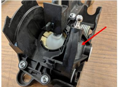
24. Using a Philips head screw driver remove the 4 screws shown below.
