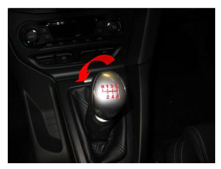
1. Start by removing the shift knob. Grab your knob and rotate it counter clockwise.
