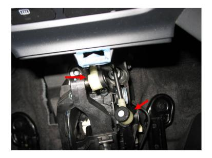
20. Slide the knurled collars towards the front of the car to remove the shifter cables from the shifter base assembly.
