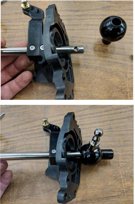
30. Apply some grease to the ball of the shifter and put the shifter cup back on to the shifter ball. Any grease will do.
