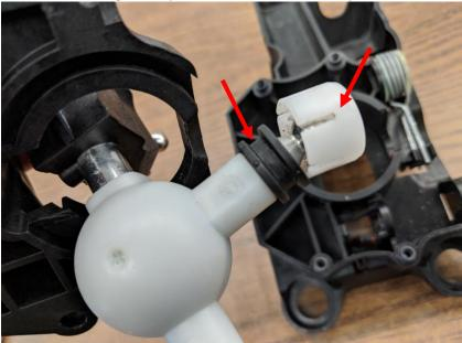
28. Orient the shifter and shifter ball cover plate as shown below. File off just a tiny bit of the edge of the shifter ball and remove from the shifter cover plate.
