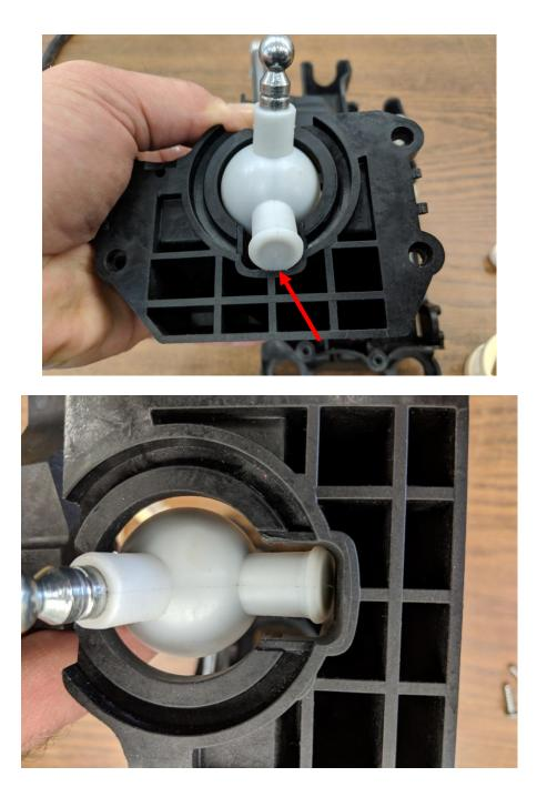
29. Put your new JBR Short Shifter threw the shifter ball cover plate as shown. Using the shifter cable actuator pin included with your kit, slide the ball onto the shifter shaft and tighten the pin using a small crescent wrench. Loctite can be applied to the threads of the shifter cable actuator pin.
