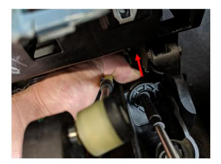
21. Remove the four 8mm bolts securing the base of shifter. There are two in the front and two in the rear of the shifter. Remove the entire shifter assembly from the vehicle.
