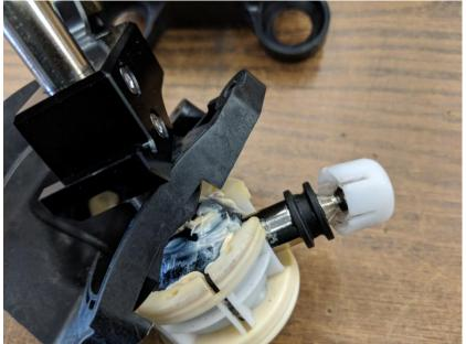
32. Using needle nose pliers, lift the centering spring and re-install the shifter cup in to the base of the shifter. Re-install the four screws.
