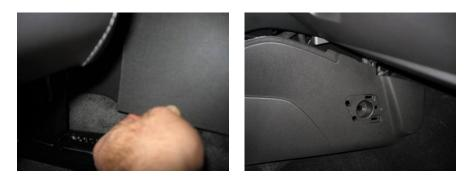
9. Using a 7/32" or 5.5mm socket, remove the three screws shown below.
