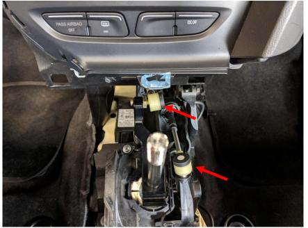
36. Remove the OEM reverse lock-out clip and replace it with the JBR reverse lock-out clip included with your kit.
