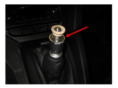
3. Remove the shift boot surround by either slipping a trim tool between it and the base of the console or using your hands. It is held in place by four clips that will need to be popped apart. Some effort is required to separate it. Do not bend the surround too much.
