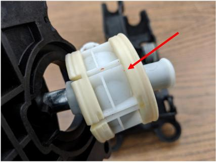
27. Remove the rubber bushing and cap from the shifter actuator pin.
