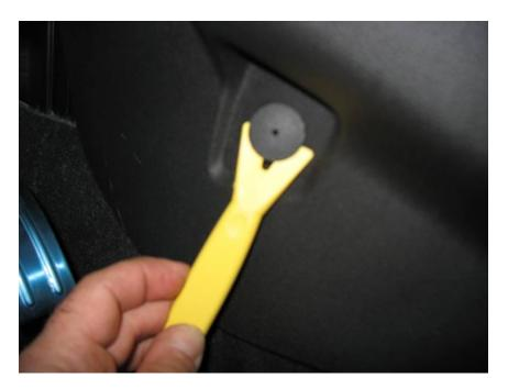
6. Separate the rear lower portion of the kick panel from the main portion of the console. Then begin separating it by moving up and towards the front of the vehicle. Separate it completely from the adjoining change cup but do not remove it completely from the vehicle.
