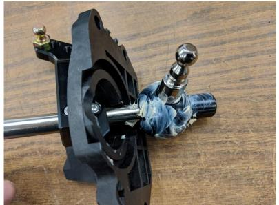
31. Put the rubber bushing and cap back on to the shifter cable actuator pin.
