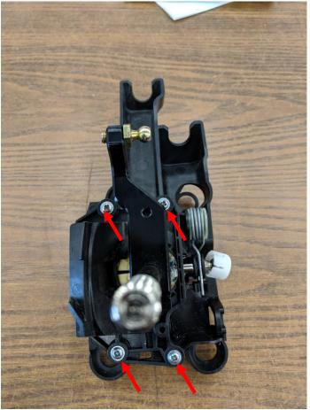
33. Put the secondary shift cable assembly arm back on to the shifter base and tap the pin in until it's flush.
