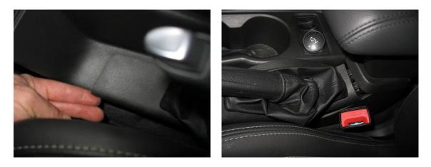
14. Pull the boot inside out and slide boot and cover off the emergency brake. Return the boot to right side out for reinstallation later.
