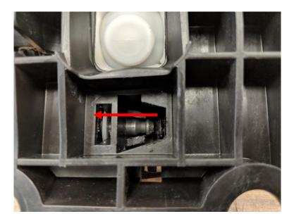
23. Remove the secondary shift cable arm from the shifter base.
