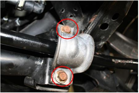
4. Apply one packet of grease to the inside of each bushing. Slip the bushing over the sway bar outboard of the lateral collar and place the bracket over the bushing as shown.
