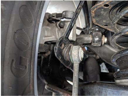
3. Disassemble one of end links and thoroughly grease the rod ends using good quality synthetic bearing grease. Failure to thoroughly grease the rod ends will lead to pre-mature failure and void the warranty.
