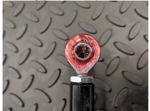
4. Install the upper portion of the end on to the sway bar as shown. Leave loose.
