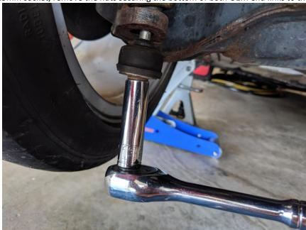
2. Using a 13mm wrench, remove the nuts securing both OEM end links to the sway bar.
