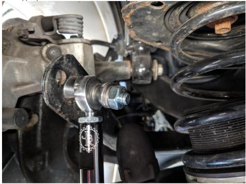
5. Install the lower end link mounting bracket so the vertical mounting tab is inboard angled a bit towards the rear of the car. Leave loose.
