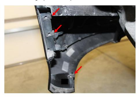
10. With a pic, clearance a hole in the fender liner larger than needed to slip one of the philips head bolt through. This is done to expose the fastener for the hole second from the top.
