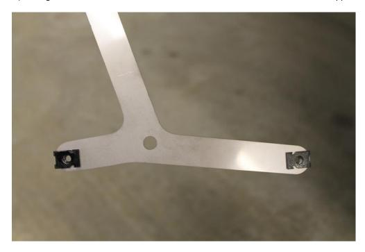
12. Using the two torx screws removed in step 7; loosely install the stainless bracket on to the rear of the mud flap. (The side with the *ST* logo)
