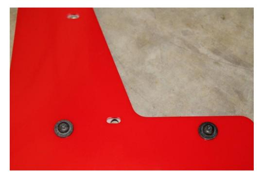
13. Place one black washer on one long bolt and slip it through the top hole in the mud flap and support bracket. Then, add one 5/8" long black nylon spacer and two 1/2" long black nylon spacers.
