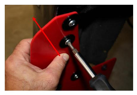
18. Tighten the remaining two philips head bolts and the two torx screws.
