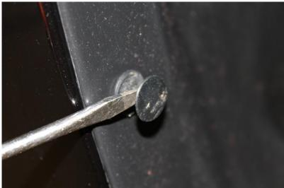
2. Pull the inner fender liner away from the fender and install 3 metal edge clips over the tabs in the fender as shown. Put the fender liner back in place.
