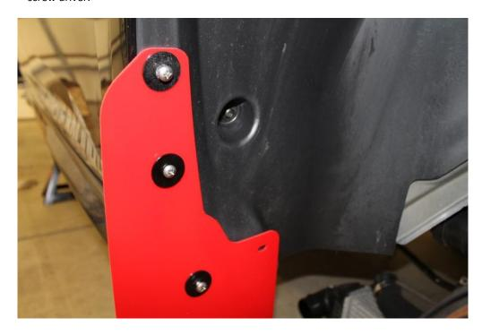
5. Next, using a drill and ¼" drill bit, drill through the remaining hole in the mud flap and through the fender liner.
