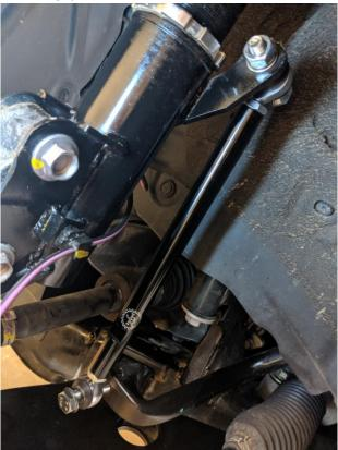
5. Adjust the length of the end links as needed and tighten the jam nuts.
