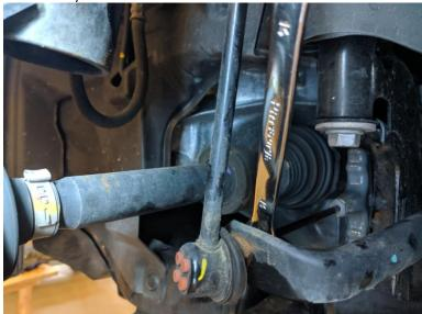
3. Using a 13mm wrench and an allen wrench if necessary, remove the nuts securing the top of both OEM end links to the strut.
