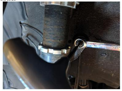
4. Disassemble one of end links and thoroughly grease the rod ends using good quality synthetic bearing grease. Failure to thoroughly grease the rod ends will lead to pre-mature failure and void the warranty.
