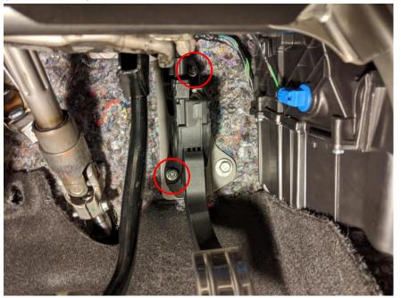
2. Using the nuts removed in the previous step; install your new JBR Throttle Pedal Spacer.
