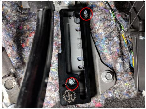
3. Using the 2, 6mm bolts, lock washers and flat washers provided, re-install the throttle pedal assembly on to the throttle pedal spacer.
