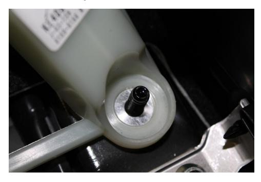
10. Place one of the 4 included washers on each of the studs, replace the nuts removed in step 7 and tighten all for nuts.
