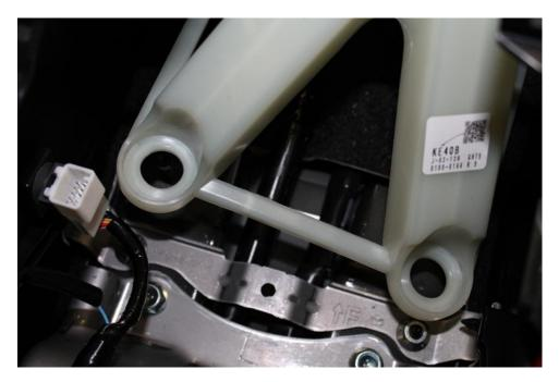
9. Place your new JBR solid shifter base bushings over the studs that secure the shifter cage to the floor with the small diameter side up. Then set the shifter cage down on to the bushings being sure the bushings index in to the base of the shifter cage.
