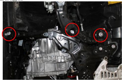
8. Using a 14mm socket remove the 4 bolts, 2 on each side, that secure the OEM bushings and brackets to the top side of the sub-frame.
