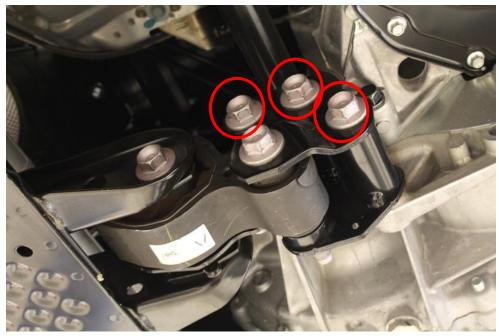
4. Remove the two bolts using a 17mm socket then, remove the mount from the top side of the rear mounting bracket.
