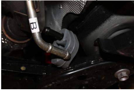
7. Support the sub-frame using a jack or jack pole and remove the 3 bolts on either side that secure the sub-frame to the chassis using a 17mm and 19mm socket. Then lower the sub-frame until it hangs with no support.
