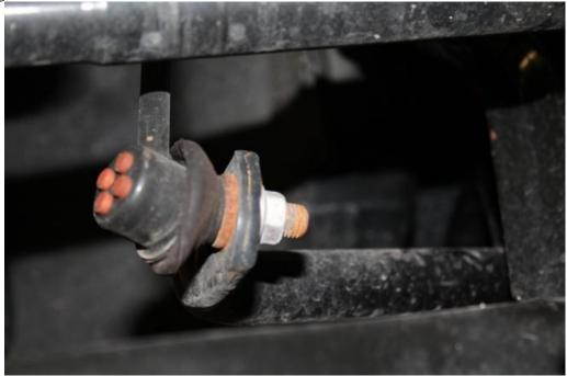
6. Remove the exhaust hanger from its rubber mounting bushing.
