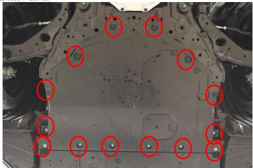
3. Remove all the bolts and push lock pins securing the heat shield using a 10mm socket and a flat head screw driver.
