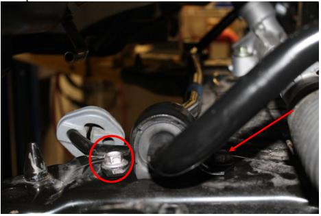
9. Remove the sway bar from the vehicle by moving it back, sliding it towards the driver's side, up and over the driver's side axle. Rotate it clockwise while pivoting it towards the rear and driver's side of the vehicle. Once it's parallel with the driver's side, remove it from the vehicle. The next series of pictures illustrate the removal and installation process.
