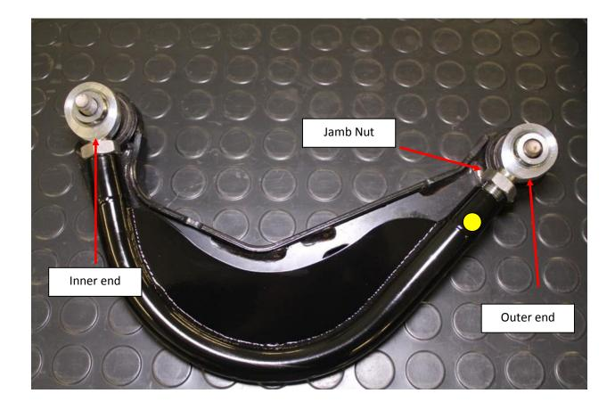
13. With the arm properly adjusted, reinstall the arm in the vehicle with the outer end closest to the wheel. Install the 2 smaller spacers on either side of the rod end closest to the wheel. Use a 17mm wrench to tighten the bolt.
