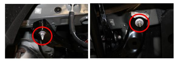
9. Next, remove both nuts securing the <u>passenger</u> side sub-frame to the chassis and lower the subreframe as far as possible. The end of the studs should no longer be visible.
