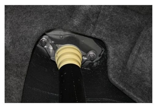
4. Using a 14mm box wrench, remove the nut securing the end link to the lower control arm. The use of a 5mm allen wrench may be necessary.
