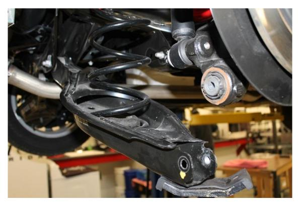
8. Using a 17mm socket and extension, **loosen** the 2 nuts on the <u>driver's</u> side securing the subframe to the chassis. Leaving the nuts in place held by only a few threads.
