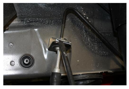
6. Using a 17mm socket remove the lower control arm bolt.
