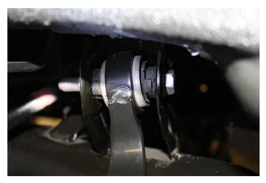
11. Using a 17mm wrench remove the outer camber arm bolt and remove the camber arm from the car.
