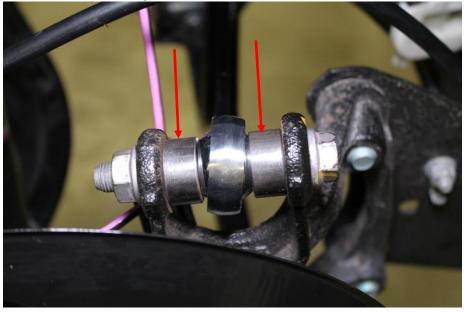
14. Install the 2 larger spacers on opposite end on either side of the rod end. Use a 17mm wrench to tighten the bolt.
