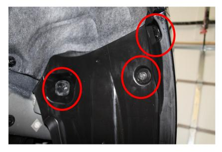
2. Remove the 2 philips head screws securing the remainder of fender liner from below and remove the fender liner from the vehicle.
