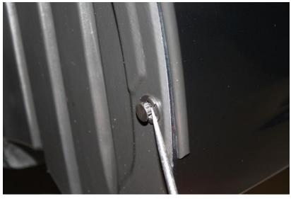
2. Pull the inner fender liner away from the fender and install 3 metal edge clips over the tabs in the fender as shown. Then, put the fender liner back in place.
