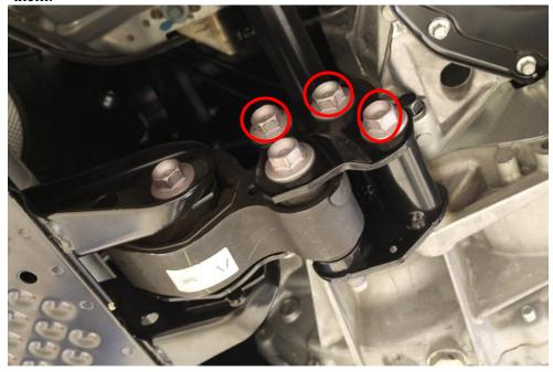
4. Remove the two bolts below using a 17mm socket then, remove the mount from the top side of the rear mounting bracket.
