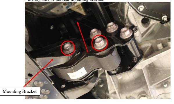
5. Install the mount from the top side of the mounting bracket as show below. Loosely install the 2 bolts removed in step 4. Then tighten the 3 bolts loosened in step 3 to 45ft/lbs and then the remaining two to 45ft/lbs.
