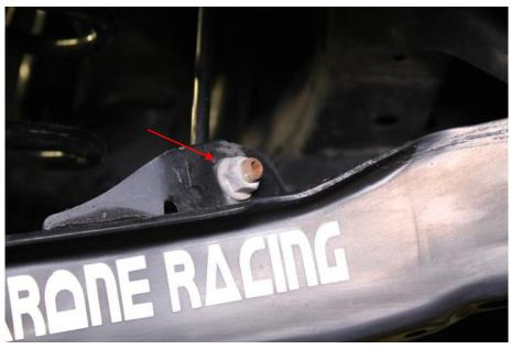
2. Using a 19mm wrench, remove the lower shock nut.
