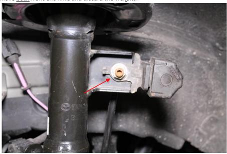
2. Using a pair of needle nose pliers squeeze the tabs and remove the clip securing the upper ABS sensor wire.
