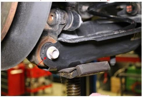
4. Install the adjustable spring perch in to the lower control arm, place the large disc below. Thread the bolt up into the upper portion of the spring perch. Then, tighten using a 22mm socket to 50-55 ft/lbs.
