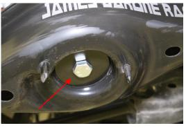
5. Using a 6" extension and a 14mm socket, remove the two nuts securing the upper shock mount.
