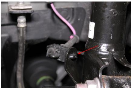
3. Using a flat dead screw driver and a pair of pliers, remove the clip that secures the brake line to the strut.
