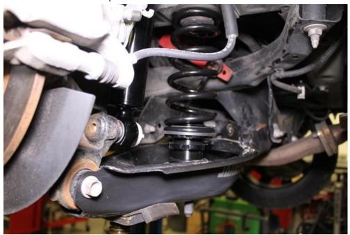
8. Place about a ½ to ¾" of upward pressure on the rear spring using the jack, adjust the shock length and reinstall the 2 nuts removed in step 5. Tighten the lower locking collar on the shock and tighten the upper buts to 35-40 ft/lbs
