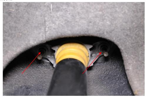
6. Install your new JBR shock on to the lower mount only at this time and tighten to 45-50 ft/lbs.
