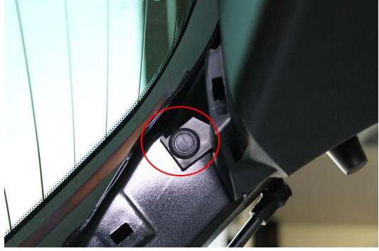
5. Remove the handle trim by pushing up and pulling out.
