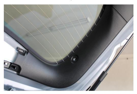
4. Next, use a flat head screw driver to remove the plastic push near the latch assembly and the two on either side.
