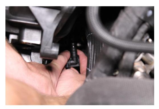
5. Next, swivel the connector removed in the previous step towards the passenger side and connect the hose with the straight end provided with your kit to it.
