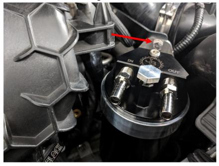
10. Put the hose clamps included with your kit on each of the hoses. Connect the hose from the intake manifold to the OUT port. Connect the hose from the PCV to the IN port. Tighten with a flat head screw driver.
