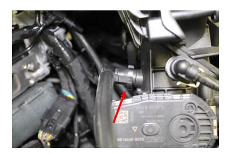
7. Route the hoses around the front of the vehicle with the hose with the 90 degree connector on top of the other. Secure them together with the zip ties provided.
