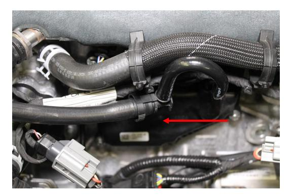
6. Connect the hose with the 90 degree end to where you removed the OEM PCV hose from the back of the intake manifold.
