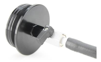
2. Apply Teflon tape to the threads of the barbed fittings. Install the barbed fittings into the IN and OUT ports of the catch can using a 14mm deep socket.
