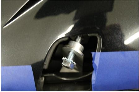
6. Hand tighten the bolt until snug, level and then tighten to 55ft-lbs using a 14mm socket.
