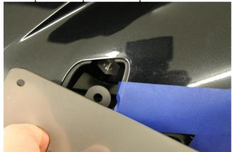
5. Place the external tooth lock washer on to the 14mm bolt, slip it through the hole in the bracket and add the aluminum spacer. Add a few drops of Loctite to the end of the bolt.
