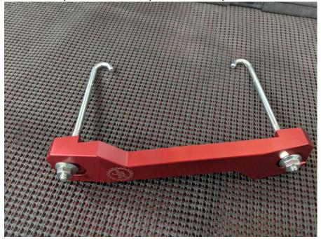
4. Install the assembly back in the car and swivel the J-hooks in place to catch the hoops at the base of the batter tray.
