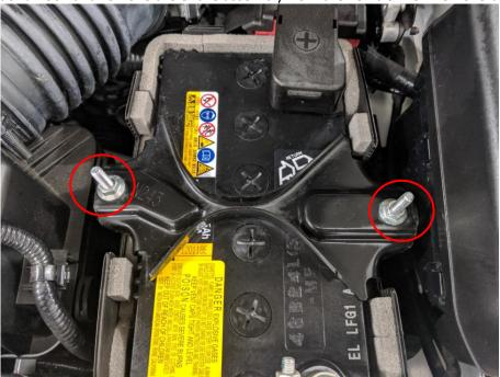
3. Install the J-hooks into your New JBR Battery Hold-Down Strap as shown.
