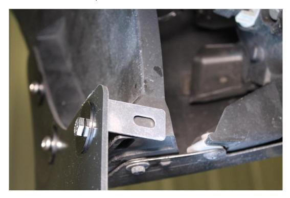
11. Align the opposite side of the angle bracket as shown, mark, and drill with the 1/8" then the 1/4" drill bit. Secure the angle bracket to the inner fender liner with a 1/2" hex bolt, lock washer and nut. Level the mud flap, and then tighten both ends of the angle bracket with an 11mm socket and an 11mm wrench.
