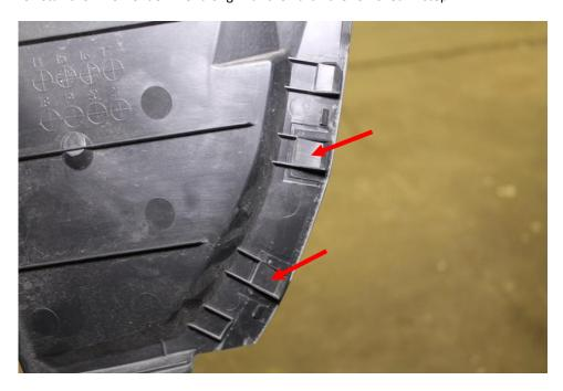
9. Place two plastic washers on two philips head bolts and thread them in to the holes in the inner fender liner. Look to the inside of the bumper and be sure the bolts are going through the tabs.
