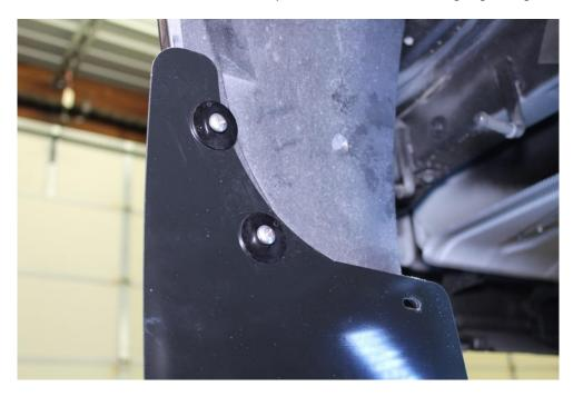
10. Next, using and angle bracket, 1/2" hex bolt, plastic washer, lock washer and nut loosely install the bracket to the mud flap as shown.
