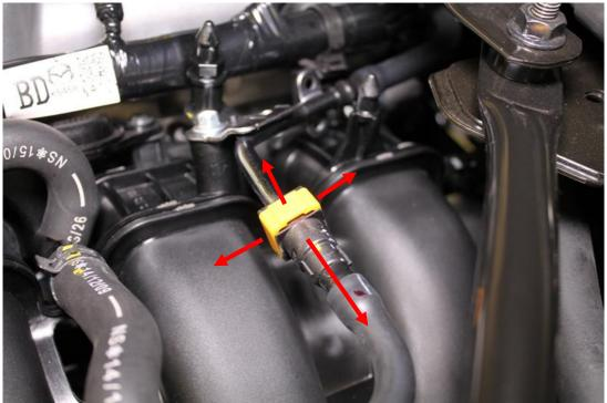
16. Using an 8mm socket, remove the bolt securing the fuel line to the intake manifold.
