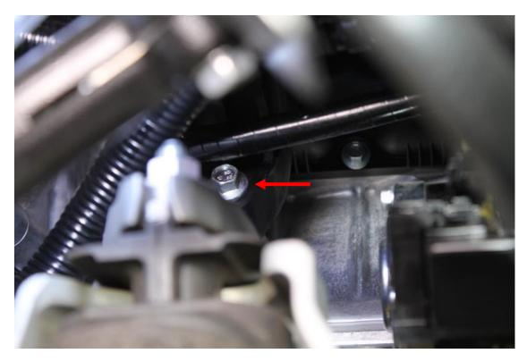
23. Now, remove the five 10mm bolts that secure the intake manifold to the head. The next three pictures show their locations. Do not attempt to remove the manifold yet.
