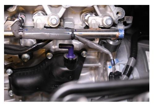
30. Attach and secure the 36" piece of hose to the PCV with one of the small hose clamp provided using a flat head screw driver.
