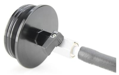
2. Apply Teflon tape to the threads of the barbed fittings. Install the barbed fittings into the IN and OUT ports of the catch can using a 14mm deep socket.
