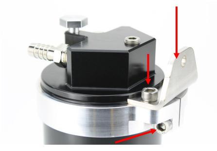
4. Using a 6mm bolt, flat washer and lock washer, attach the mounting bracket squarely to the mounting bracket already installed on the catch can. Tighten with a 10mm wrench.
