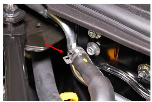
18. Using a pair of pliers, squeeze the spring clamp, slide it back and remove the vacuum hose found just off center, close to the cowl on the driver's side. Twist to loosen and then remove.
