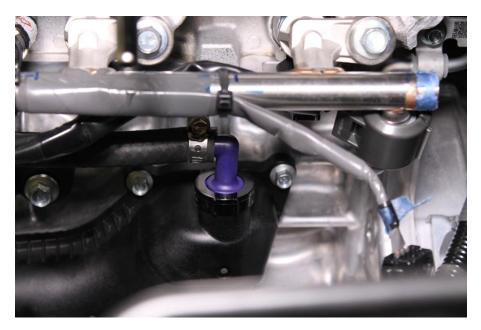
31. The hose leading from the PCV is to be routed behind the fuel rail towards the front of the vehicle.
