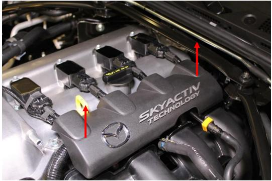
12. Using a pair of needle nose pliers, squeeze and disconnect the clips holding the wiring harness to the top of the intake manifold. There is one at the front and one at the rear of the engine.
