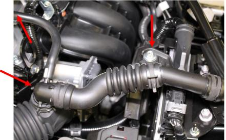
11. Pull up on each end of the fuel rail cover and remove.
