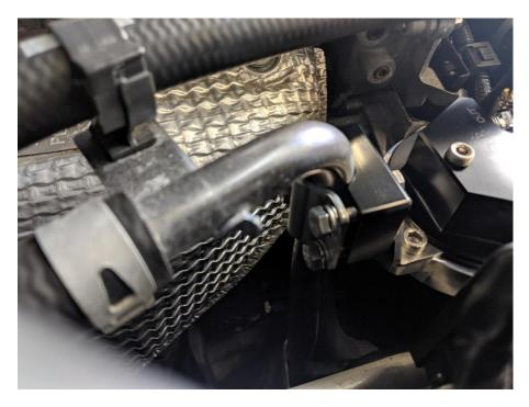
The drain hose should be routed down near the area of the oil pan drain plug
