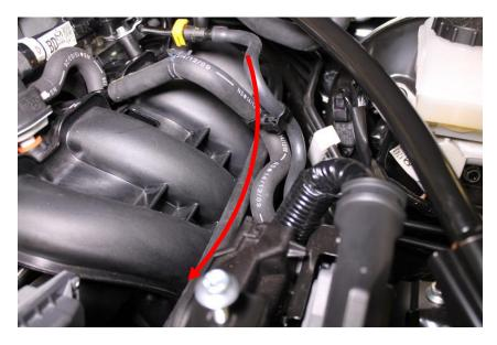
41. Secure the hose from the intake manifold to the wiring harness below the throttle body.
