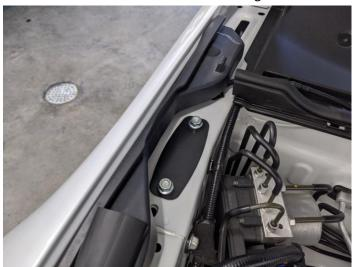
2. Using a 6mm allen wrench, install your new JBR Sill plate and tighten to 15 ft/lbs.
