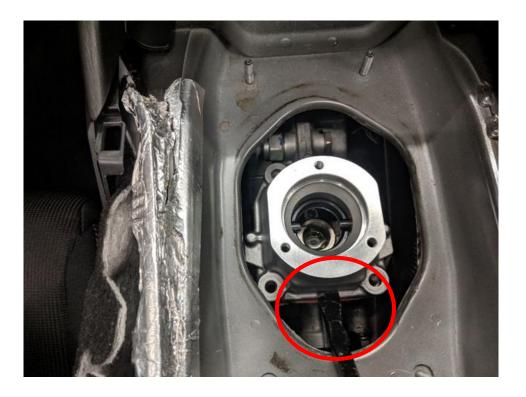
12. Using a rag and some pressure, remove the silicone sealant from the top of the transmission and the bottom of the cup removed in the previous step. Get both as clean as possible.
