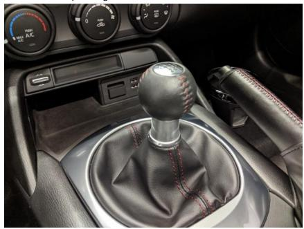
2. Remove the shifter boot bezel by hooking your fingers under the bezel in the areas by the arrows and tugging straight up.
