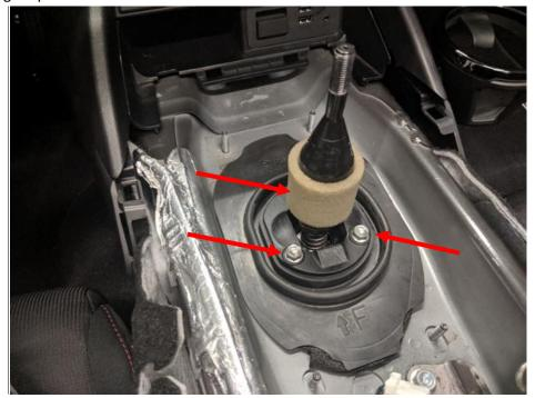
10. Using a 12mm socket and short extension remove the 4 bolts securing the upper cup to the transmission.
