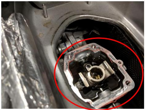
13. Put a thin film of red RTV sealant on the top of the transmission, then place the spacer include with your JBR shifter on top of the transmission being sure to line up the indexing pins.
