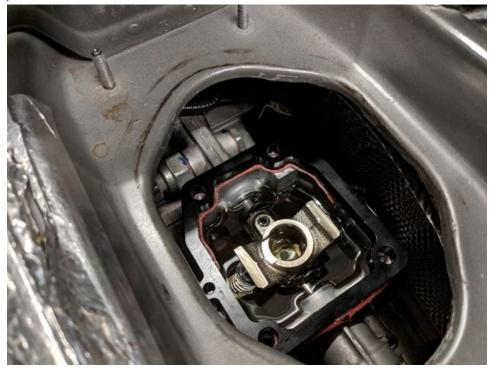
14. Put another thin coat of red RTV on top of the spacer installed in the previous step and install the upper cup removed in step 10. Using the 4, 35mm bolts include with your kit, secure the upper cup to the transmission and tighten to 14 ft/lbs with a 13mm socket and short extension.
