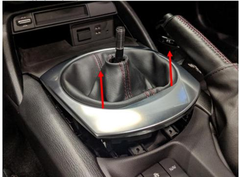
3. Remove the 2 philips head screws securing the console in front of the shifter.
