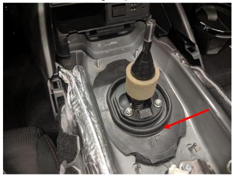
9. Remove 3, 10mm bolts holding the shifter into the top of the transmission and lift the shifter straight up and out.
