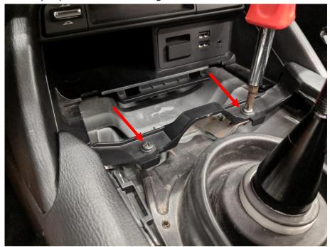
4. Remove the console by hooking your fingers under each edge of the console and tugging up at the same time from each side in the area by the arrows.
