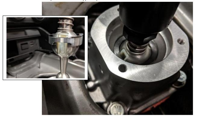
17. Place the upper cup cover and cup cap over the shifter and on to the upper cup of the transmission. Use the 3 6mm x 25mm bolts, flat washers and lock washers included and tighten to 8 ft/lbs with a 10mm socket.
