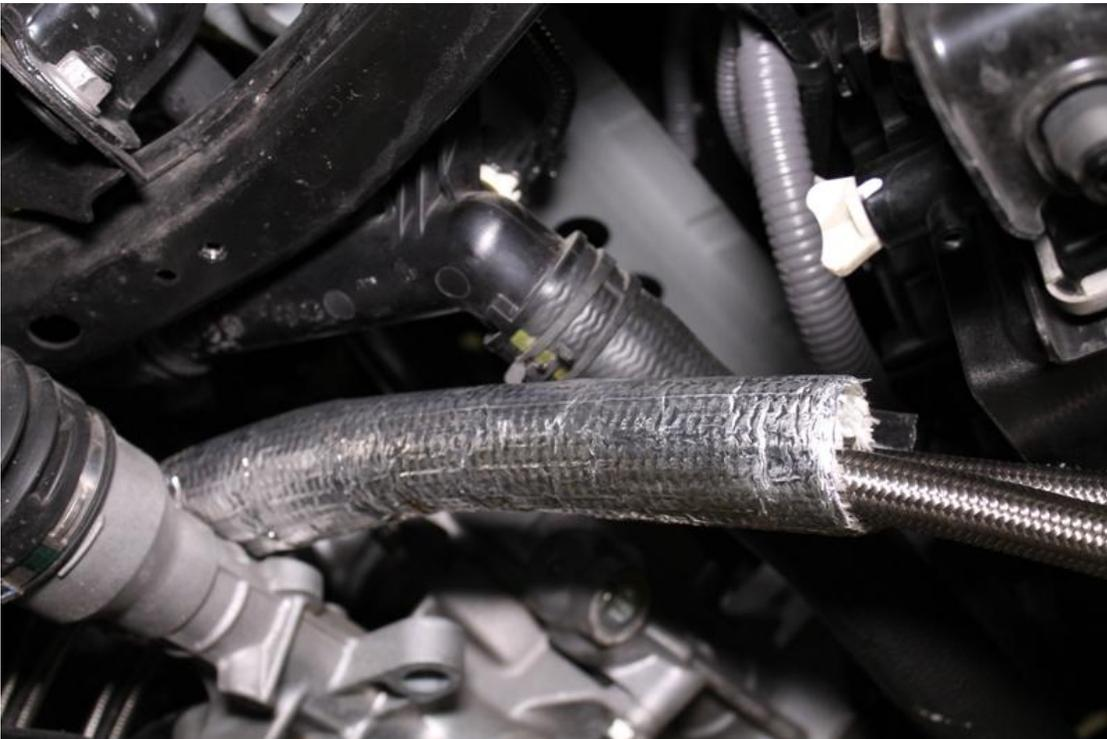
12. Using 2 large crescent wrenches, install and tighten the braided lines on to the core.
