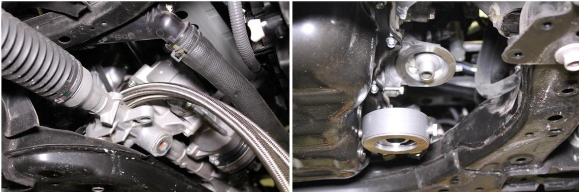
7. Using adapter plate bolt, install the adapter plate on to the filter housing.
