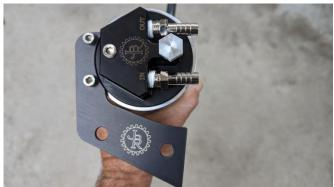
If you need to adjust the location of the mounting collar, ALL 3 socket cap bolts must be loosened.
