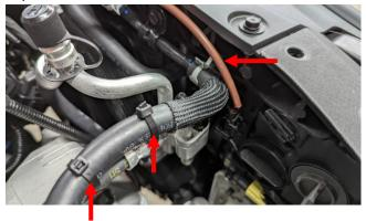
13. Disconnect the wire loom from its mounting point shown below and secure it towards the passenger side of the car as shown with one of the 5" zip ties.
