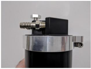
8. Install the mounting bracket to the mounting collar included with your kit.
