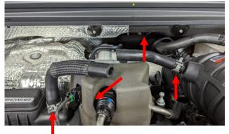
4. Apply Teflon tape to the threads of the 3/8" barbed fittings provided with your kit. Install the barbed fittings into the IN and OUT ports of the catch can using a 14mm deep socket.
