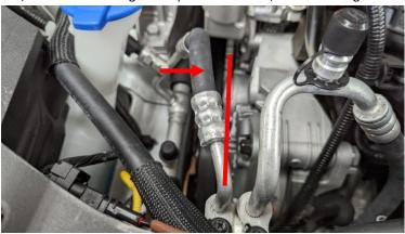
10. Disconnect the wire shown below from its mounting point on the core support.
