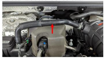
4. Using a pair of pliers, loosen the clamps and rotate the cam cover hose straight towards the front of the vehicle and rotate intake hose towords the rear.
