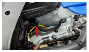
14. Remove the bolt securing the A/C line bracket to the frame. Place the round spacer included with your kit between the bracket and the frame. Re-secure the bracket with the included 35mm bolt, flat washer and lock washer. Patience is needed here. Don't drop/loose the spacer.
