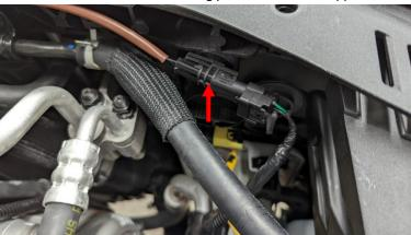
11. Remove the coolant hose from side of the windshield washer fluid reservoir. Raise it over the top of the reservoir towards the driver's side.
