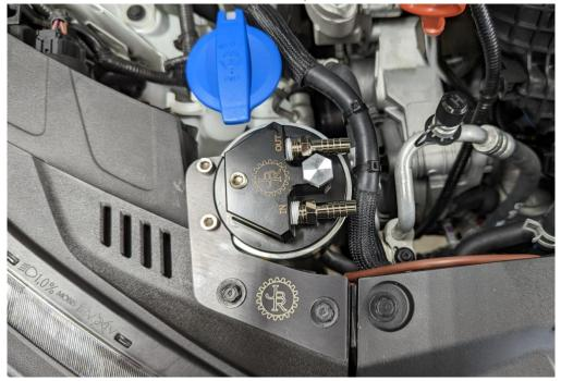
17. Remove the catch can dipstick and connect the 21" hose to the IN port on the catch can and the 30" hose to the OUT port. Secure with two of the small hose clamps and 1, 8" zip tie as shown below.
