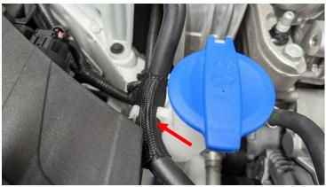
12. Secure the coolant hose ON TOP of A/C line you moved in step 9 with 2 of the 8" zip ties. Then, route the wire you removed in step 10 as shown below.
