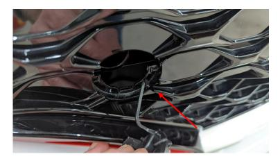
2. Install the large hex bolt and tighten to 50ft/lbs
