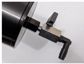
8. Apply Teflon tape to the threads of the barbed fittings provided with your kit. Install the barbed fittings into the IN and OUT ports of the catch can using a 14mm deep socket.
