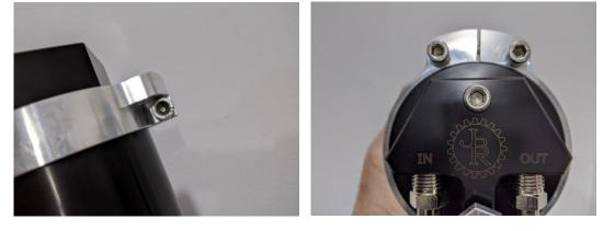
10. Tighten the mounting collar so it's just below the top edge of the catch can.
