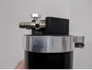
11. Install the mounting bracket to the mounting collar included with your kit.
