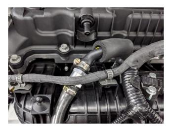
6. Use the clamp removed in step 6 and attach the other hose provide with your kit to the PCV valve.
