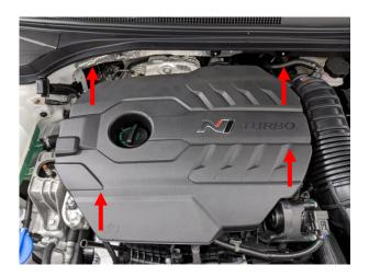
2. Un-clip and remove the air box cover.
