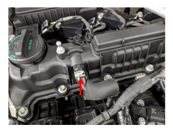
5. Attach the provided hose with the check valve to the end of the hose removed in the prior step and attach with the large hose clamp provided in your kit.
