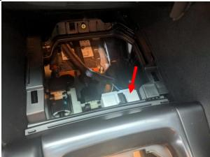
10. With the passenger side now loose and the storage shelf removed, use your hand and tug straight up in the area where the emergency brake handle cover was to loosen the driver's side of the center section of the console from the base of the console.
