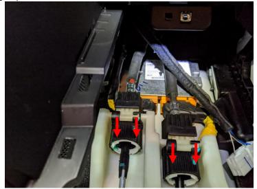
13. Using needle nose pliers, remove the clip securing the secondary shift cable. Remove the cable from the post.
