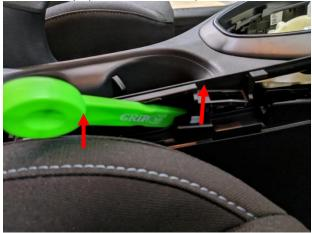
8. Remove the shelf cover in front of the shifter. Then, using a flat head screw driver and a cloth to protect the shift boot surround, pry up on each side to remove the base of the shelf.
