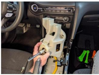
18. Using a pair of pliers, carefully grab the bushing on the bottom of the shifter and pry it off.
