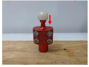
20. Loosen the four socket cap bolts a bit and slip the adapter all the way on to the base of the shifter with the logo facing the passenger side if the as if the base was installed in the car.
