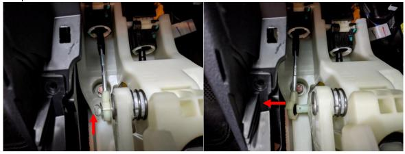
14. Using a philips head screw driver and a 10mm socket, extension and ratchet, remove the metal console support bracket.
