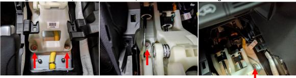
16. Raise the base of the shifter up and disconnect the primary shift cable from the shifter by spreading the wire retaining clip and pulling down on the cable simultaneously. The clip should remain on the cable end.
